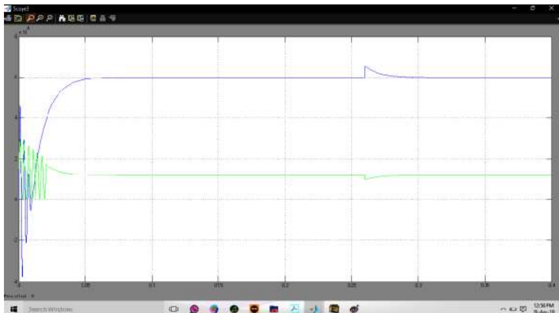
Fig. 4. The grid delivers both real (top) and reactive (bottom) power.
