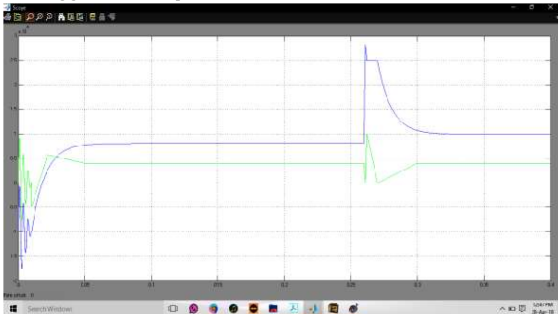
Fig. 7. Inverter 1 provides both real (top) and reactive (bottom) power..
