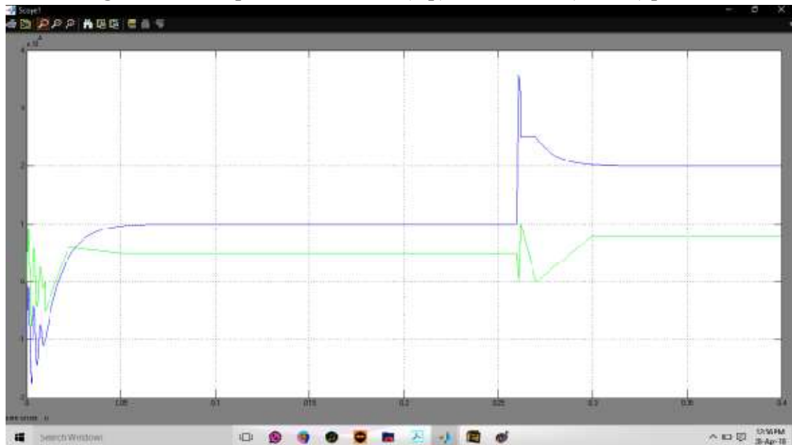
Fig. 3. Inverter 2 provides both real (top) and responsive (bottom) power.
